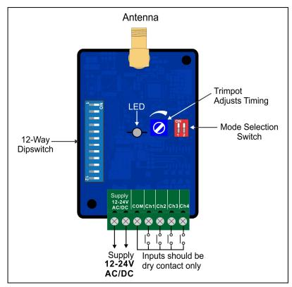
Inputs of the transmitter should be voltage free contact closure only.
